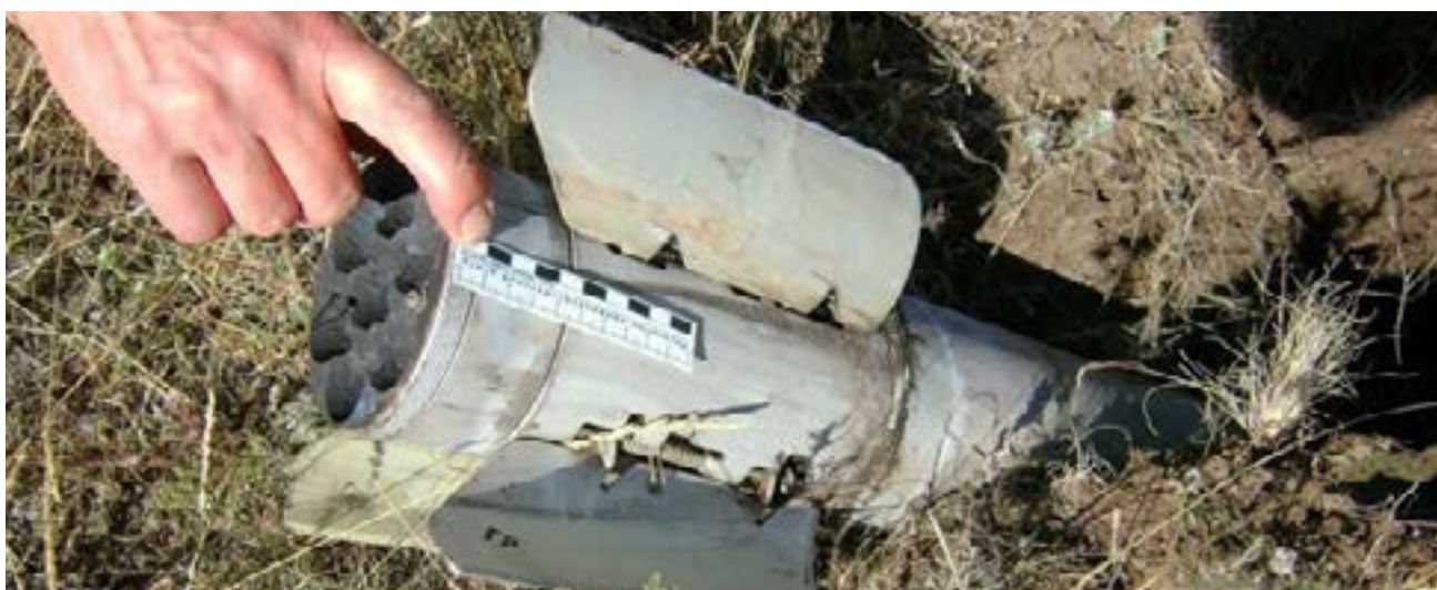
Figure 15.32. Tail section of a 122 mm rocket showing the fin release and tension system and venturi, 2012 (Source: Administration of the Sol-Iletsk urban district).
