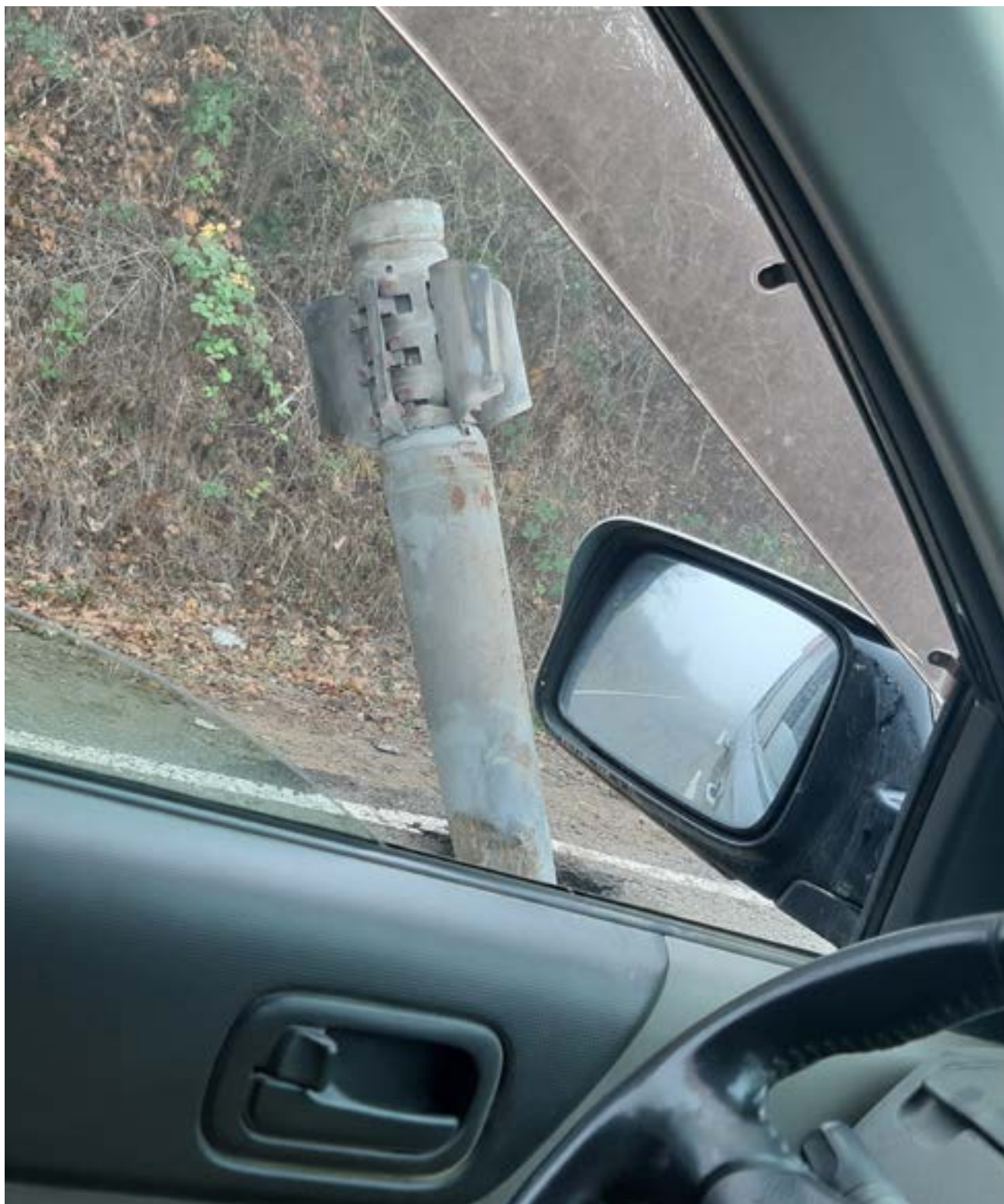
Figure 15.24. The tail section of a 9M5-series 300 mm surface-to-surface rocket buried in roadway surface, 2020 (Source: Julieta Ishkhanyan).
